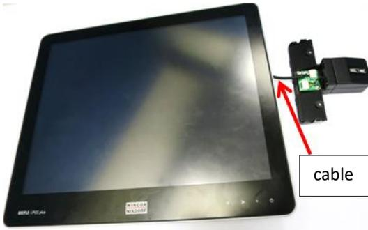
Attach the cable connector to the 2D Barcode Reader.
