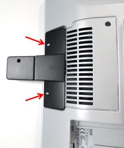
And, fasten the Torx screws onto the 2D Barcode Reader
