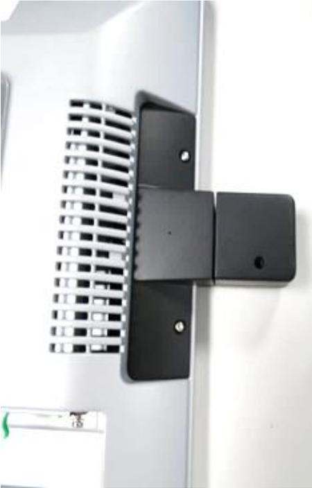
fitting the 2D Barcode Reader in place and putting on the two Torx screws.
