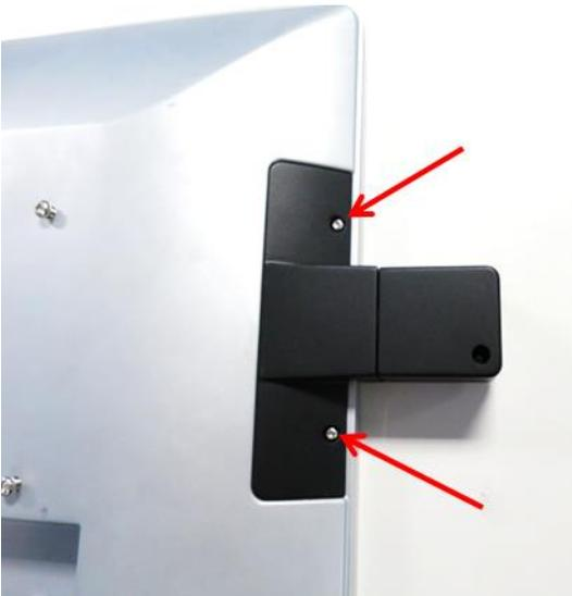
And, fasten the two Torx screws onto the 2D Barcode Reader.
