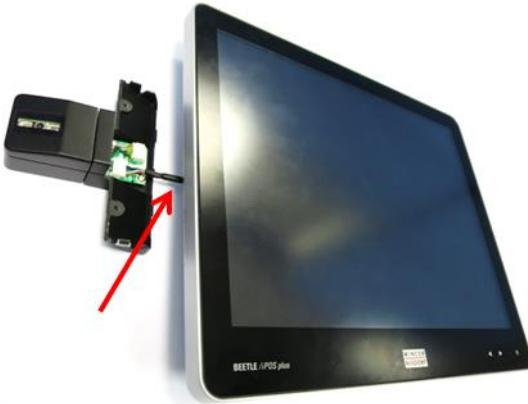
Attach the cable connector to the 2D Barcode Reader.
