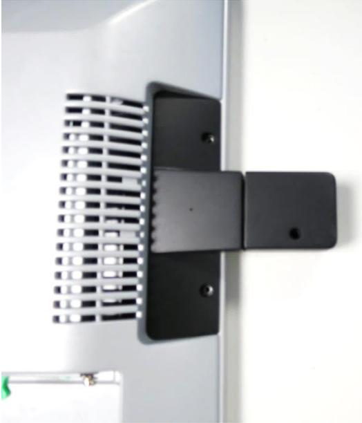
Then, fit the 2D Barcode Reader in place at the back of the display.
