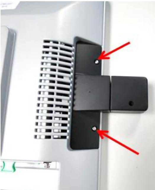
And, fasten the two Torx screws onto the 2D Barcode Reader.
