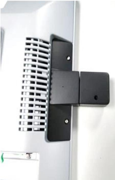
fitting it in place and putting on the two Torx screws.
