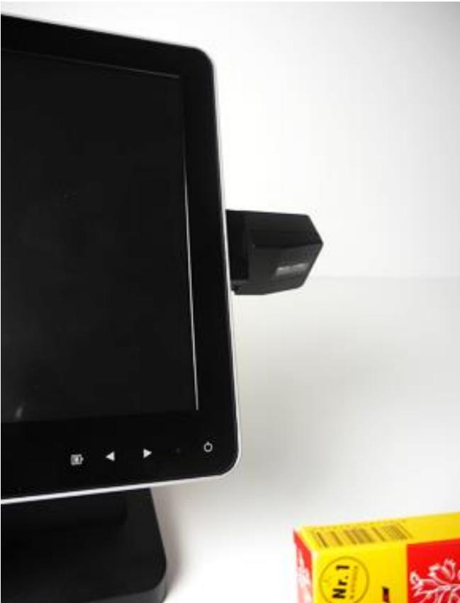
The Barcode reader is able to rotate 165 degrees clockwise and 165 degrees anti-clockwise, please see illustration below. Do not rotate the barcode reader beyond this rotating range. Doing so may damage the reader.
