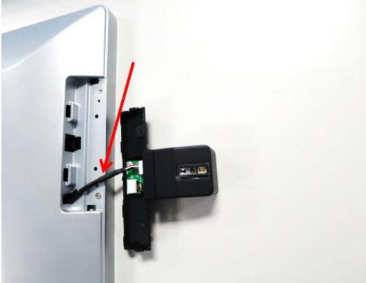
Then, attach the other end of the cable with the 2D Barcode Reader.
