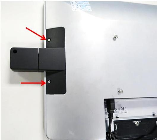
And, fasten the two Torx screws onto the 2D Barcode Reader
