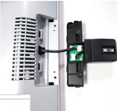
first connect the cable to the 2D Barcode Reader.
