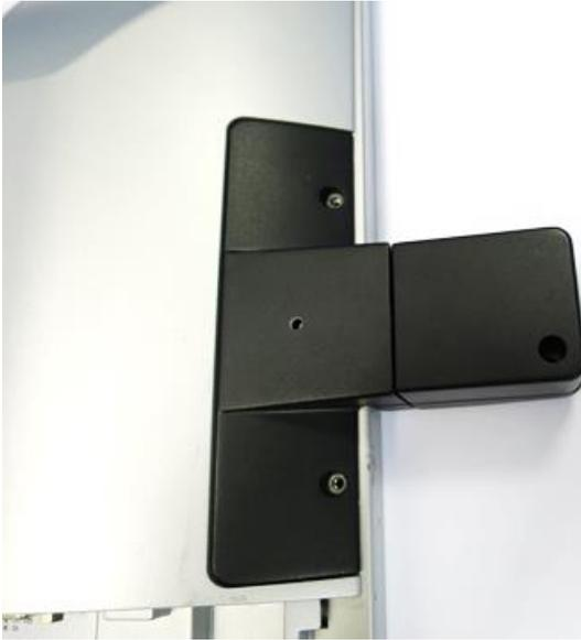
Then, fit the 2D Barcode Reader in place at the back of the display. .
