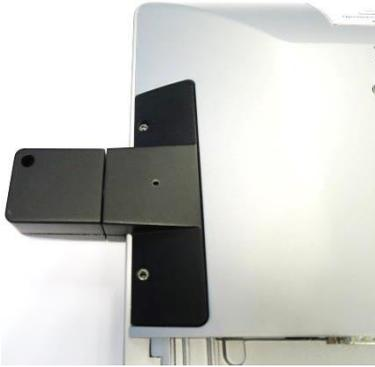
Then, fit the 2D Barcode Reader in place at the back of the display.
