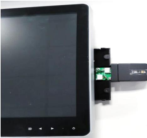
Attach the cable connector to the 2D Barcode Reader.
